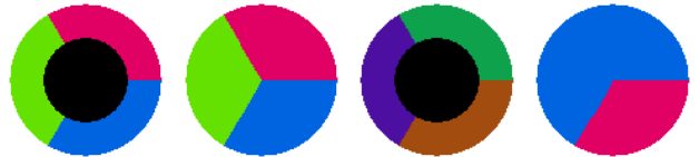
Figure 5: Three-class inpainting problem. Left to right: input with inpainting region marked in black, exemplary result, input corresponding to the “inverse” variant, exemplary result. The “inverse” variant has many equally good minimizers.
